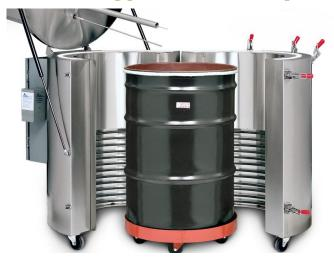
Place a 55-gallon open top drum onto the drum dolly. Transfer wastewater into the drum to within 6-8 inches of the top. With the evaporator in full open position, roll the drum into the evaporator. Wrap the rope gasket around the drum so that a positive seal will be made when the clamshell walls are closed and secured.
