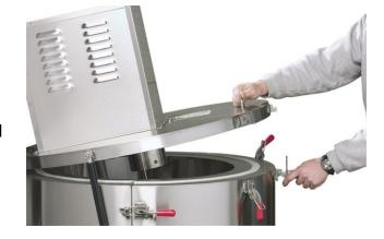
Close and secure the clamshell walls and lid with the latching handles.
