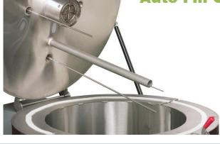
The ENCON DE-2 Drum Evaporator can be modified to run in the auto-fill mode (optional high-level probe required). The ENCON DE-4 only operates in auto-fill mode. This mode requires plumbing from a feed pump to the inlet on the top of the evaporator lid. This allows the automatic and continuous refilling of the evaporator between the height of the two level probes until either the high temperature set point is reached or there is no longer water to be processed in the feed tank.
